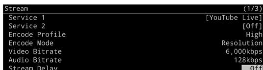
2. Turn the [VALUE/CURSOR] knob to set the streaming delay time, and then press the [VALUE/CURSOR] knob.
