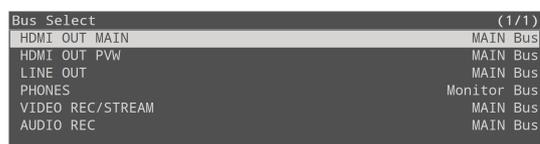
2. Turn the [VALUE/CURSOR] knob to select the output jack/connector to which the audio bus is assigned, and then press the [VALUE/CURSOR] knob.
