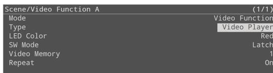
4. Turn the [VALUE/CURSOR] knob to select the function to assign to a button, and then press the [VALUE/CURSOR] knob.
