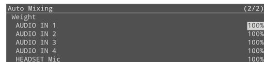
2. Turn the [VALUE/CURSOR] knob to select the audio to which the setting the priority for volume distribution (Weight), and then press the [VALUE/CURSOR] knob.
