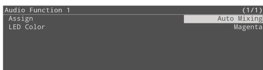
2. Turn the [VALUE/CURSOR] knob to select the function to assign to a button, and then press the [VALUE/CURSOR] knob.
