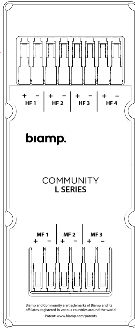
MF/HF Input Panel LVH-900/AP
